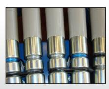
24 VDC roller drives are fully enclosed powered rollers: one drive roller can drive up to 3m of conveyor when slaving adjacent rollers.
