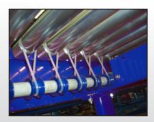
Lineshaft powered roller conveyors employ drive bands to transfer power from a common drive shaft.
