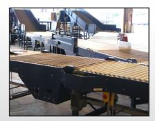
Live roller conveyors use a narrow belt underneath to drive the rollers.
